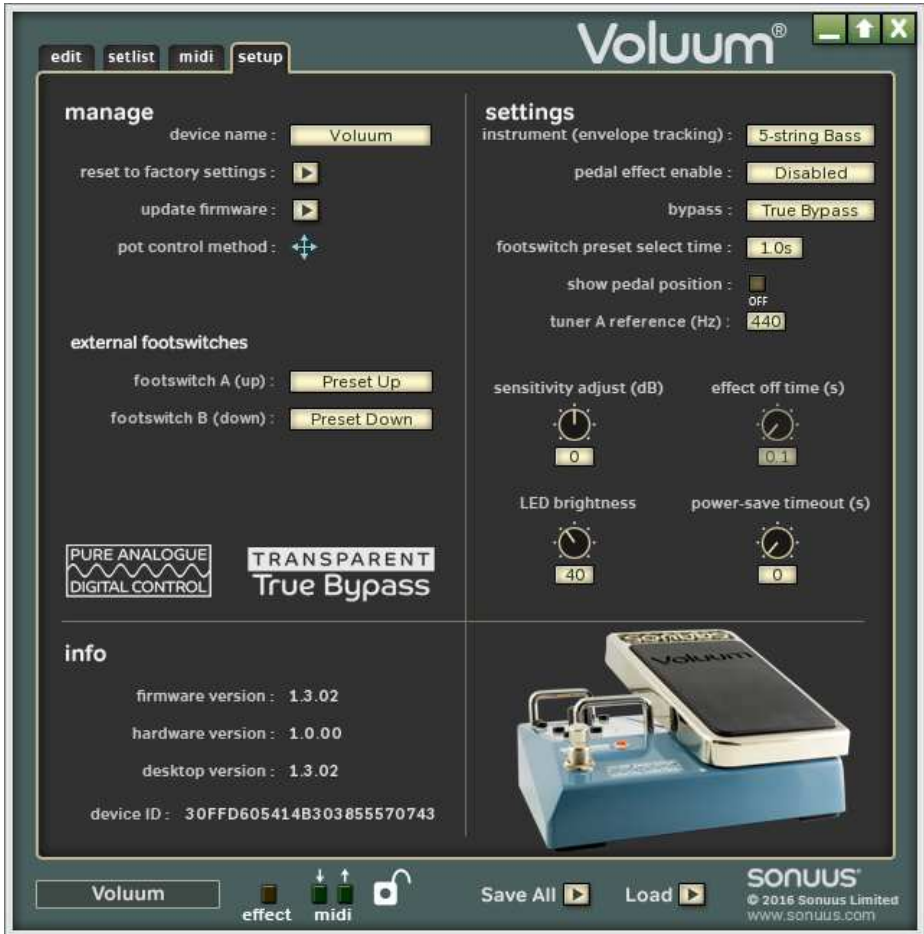
Figure 8: The setup tab lets you change global settings, manage your device and gives information on the version of hardware and firmware in your Voluum .
