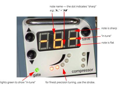
When you tune, the note being played is shown on the display. The closeness to being in-tune for the note is shown in several ways:
