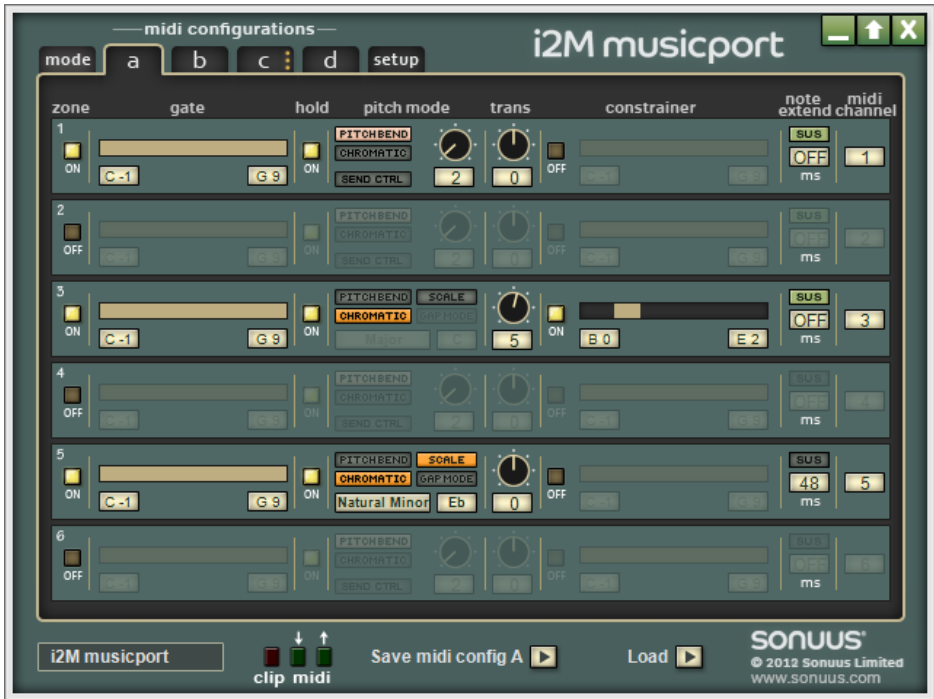
Figure 6: MIDI Configuration / Zones. The currently active MIDI Configuration is highlighted so you know if the one you are editing is currently active or not
