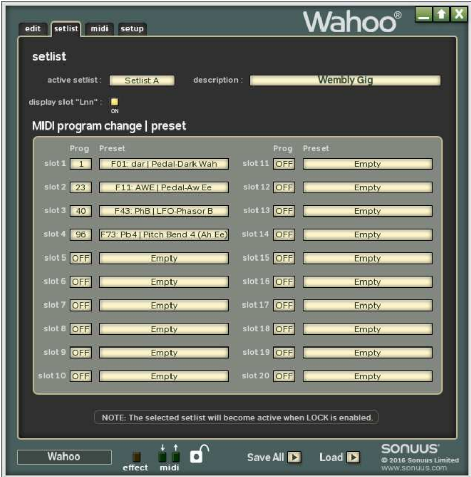
Figure 10: The setlist tab lets you create setlists: a list of only those presets that you want to be available when you lock the Wahoo — perfect for playing live.
