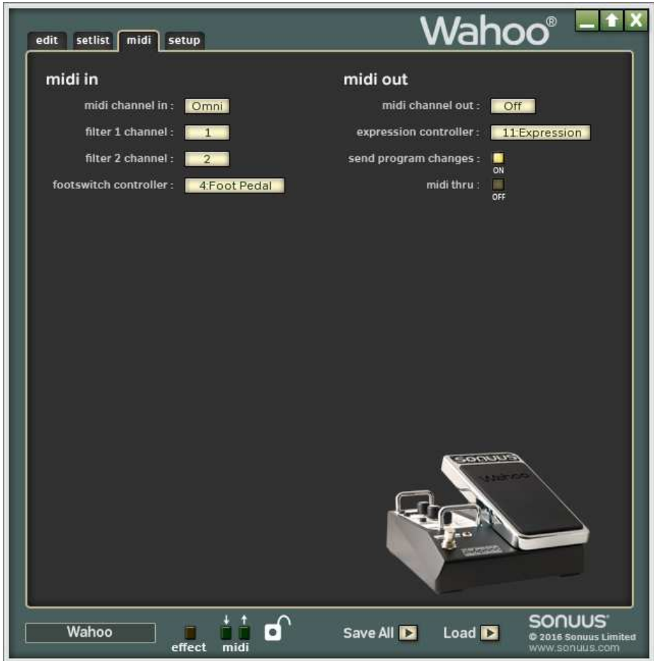
Figure 11: The midi tab lets you configure how MIDI is sent and received over the USB connection of the Wahoo .
