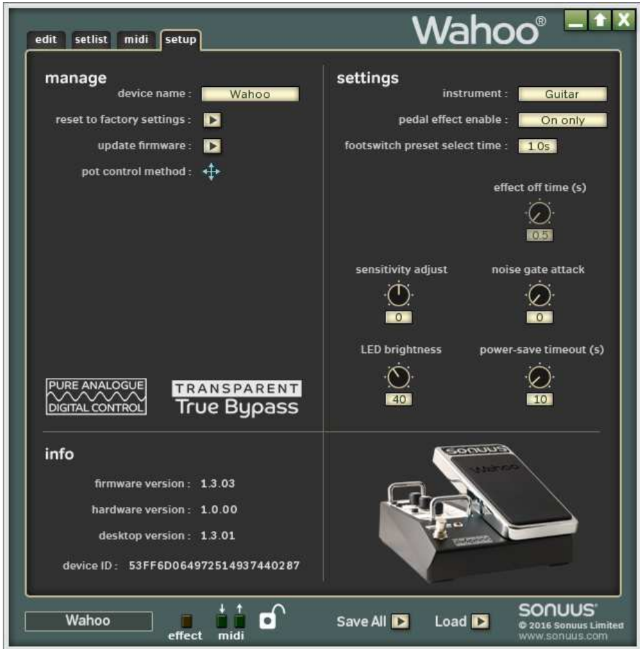
Figure 12: The setup tab lets you change global settings, manage your device and gives information on the version of hardware and firmware in your Wahoo .
